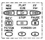
TV/Video Button — Press the TV/VIDEO button to select desired input for Main Picture or PIP frame
