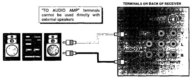
Adjustment - When an audio amp is connected to "TO AUDIO AMP" terminals
