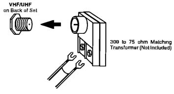
Cable Connection – For reception of cable channels, connect the cable supplied by your local Cable company Antenna Mode must be set to CABLE (Refer to Antenna Mode section)
